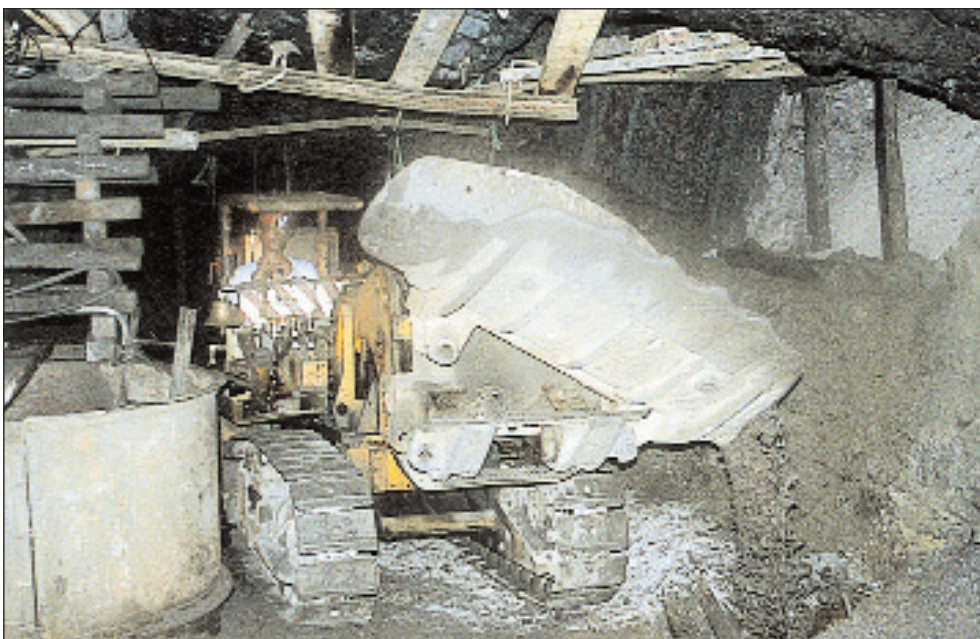
Side Discharge Loader (S.D.L.) in Operation underground Balaghat Mine
